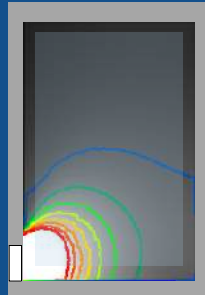
Daylit area \geq 21\% Window 1,07x2,8 W/floor = 1:8
