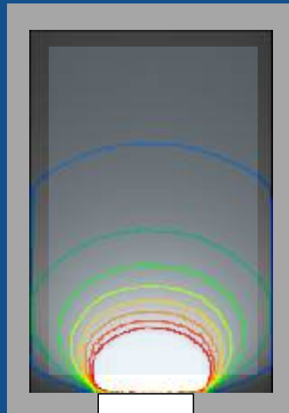
Daylit area \geq 41\% Window 1,73x1,73 W/floor = 1:8
